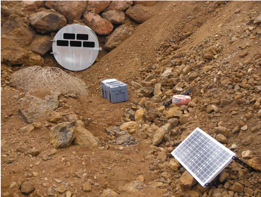
Setup of monitoring equipment at MW-AR-01 showing recording equipment (in grey box) and solar power supply.
