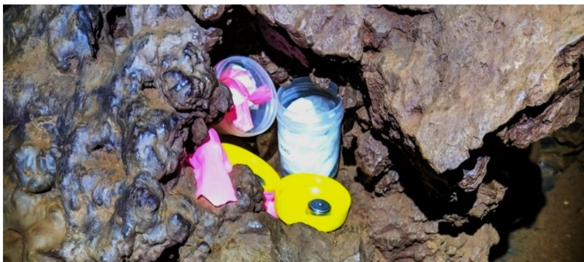
Plate 4.1: Hydrochron (DS1923) temperature and humidity loggers at CO-CA-03
